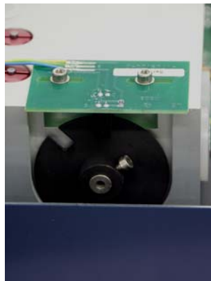
Fig. 6. Marker PCB located on top of the LC 100 motor/gearbox.
